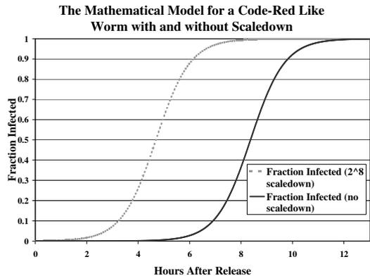
**Figure 4: The effect of scaling down the mathematical model for Code Red. With a  $1/2^8$  scaledown factor, the curve shifts substantially to the left because the *proportion* of the infected population at time  $t_0$  is larger**
