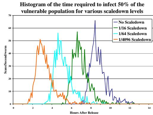
Figure 8: A histogram of 1,000 simulation runs for Code Red without scaledown, with a  $1/2^4$ , a  $1/2^8$ , and a  $1/2^{12}$  scaledown factor. The histogram shows the time when 50% of the vulnerable systems are infected.
