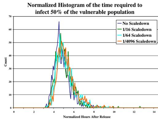
Figure 9: A histogram of 1,000 simulation runs for Code Red without scaledown, with a  $1/2^4$ , a  $1/2^8$ , and a  $1/2^{12}$  scaledown factor. Unlike the previous histogram, here we have shifted the different histograms so that  $t_0$  is equivalent.
